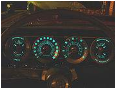
1966 Dodge Charger instrument panel with electroluminescent lighting. Chrysler began building cars with EL panel lighting for the 1960 model year
