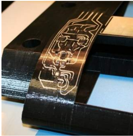
UAV wing with strain sensor
